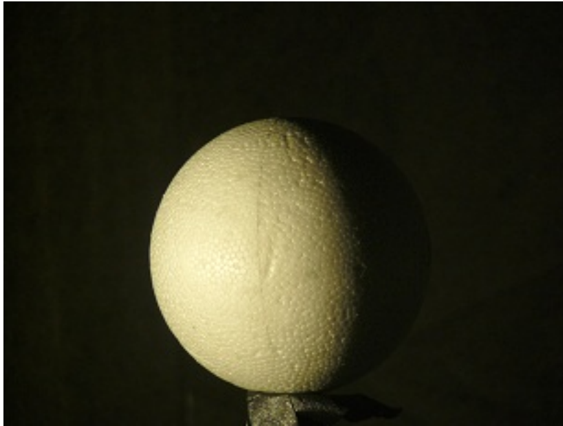
Figure 3.9: Styrosphere target used to model the sunlight scattering off of Earth. The target is illuminated by a movable broadband projector lamp.
